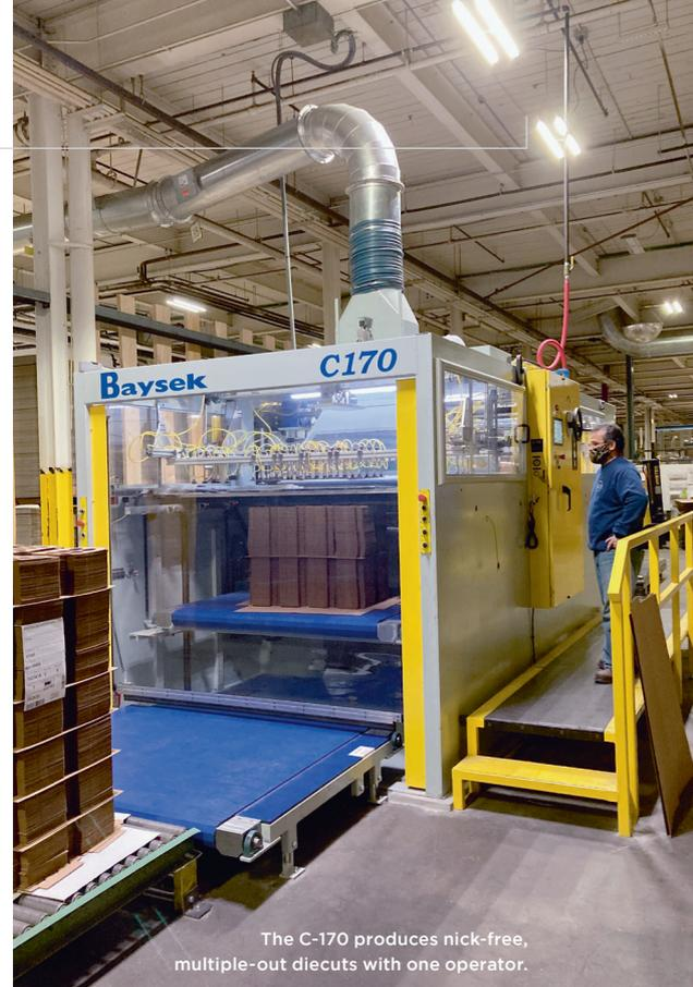
The C-170 produces nick-free, multiple-out diecuts with one operator.
